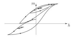
Figure 1: Hysteresis in ferromagnetism.
