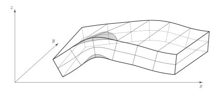
Figure 3. A plate section with grey plasticized zone.
