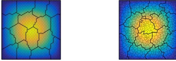
Fig. 4: Solution with virtual elements for hexagonal (left) and irregular (right) meshes and constant coefficient \rho = 1 .
